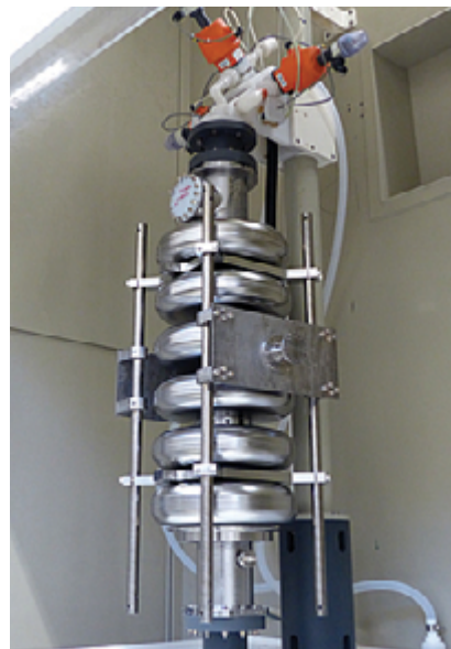
An ESS niobium cavity prototype being prepared for testing in the lab at IRFU
