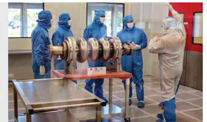
A high-beta cavity assembly in the ISO 5 cleanroom at IRFU in Saclay, France.
