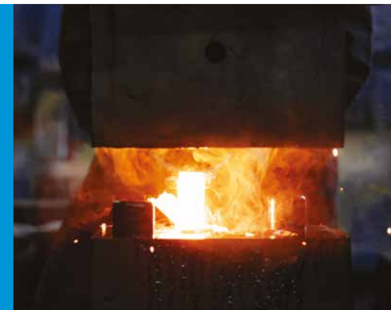
A hydraulic hammer shapes the hot material as it rapidly cools in a forge – a commonly used process in the production of machine parts. ESS will have a furnace and hammer inside the BEER instrument, enabling real-time neutron monitoring of the microstructures in the material as it is reshaped and rapidly cooled into its final form. This allows researchers to control the final material properties.
