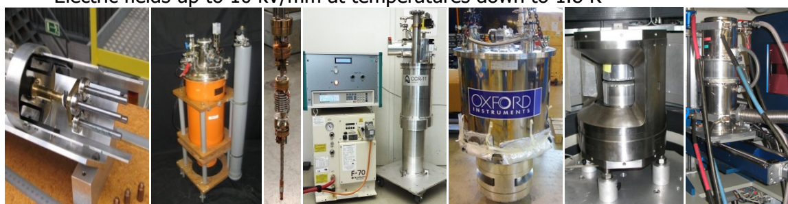
Figure 17 From left to right: multi low temperature sample changer, orange cryostat, closed cycle cryostat, cryomagnet, pressure cell, high temperature furnace. (Pictures PSI, ILL, FRM2).
