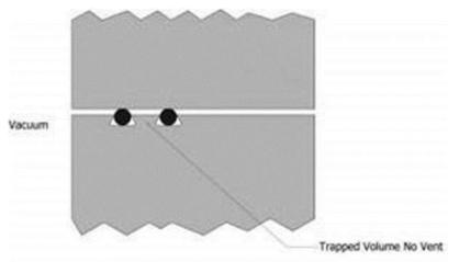
• Trapped volumes caused by unvented single or double dovetail o-ring groove designs.
