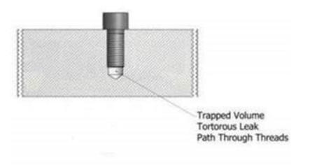
• Trapped volumes caused by unvented double o-ring seal designs.
