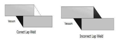
The correct style lap weld uses a full continuous weld at the vacuum side. If more structural strength is required, a skip weld can be added to the non-vacuum side. The incorrect style lap weld uses two continuous welds on both the vacuum and non-vacuum side or a single weld on the non-vacuum side leaving a trapped volume for gas and contaminants.
