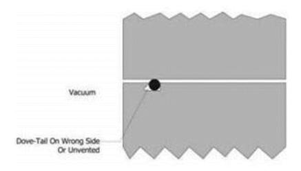
• Trapped volume caused by incorrect weld design
