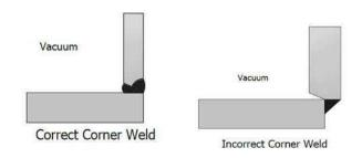
The correct style corner weld has the two sides that meet to form the corner flush with each other, and uses a full penetration weld. The incorrect style corner weld has one side overhanging the other at the weld joint, leaving a trapped volume for gas and contaminants.
