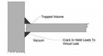
• Trapped volumes caused by uneven up of full penetration welds and lack of interior welds or braze joints.
