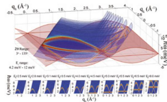
*Example of a magnon dispersion measured on a BIFROST indirect geometry setup. A BIFROST data-set is 3-dimensional: Two in-plane Q-coordinates and an energy transfer. Each set of analyzers effectively measures a 2-dimensional manifold in this space.*
