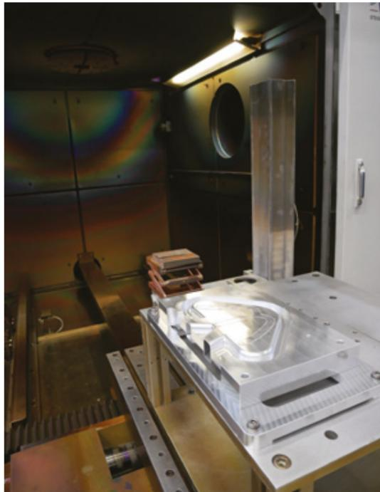
*Electron welding of the ESS low-dimensional moderator at FZJ*
