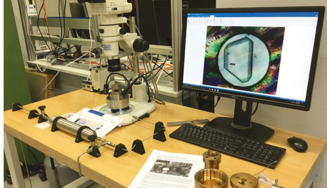
On the monitor, a single crystal of a high-pressure ice VI with growth controlled remotely by gas pressure. On the table, components of the ESS-designed Diamond Anvil Cell made from BeCu.
