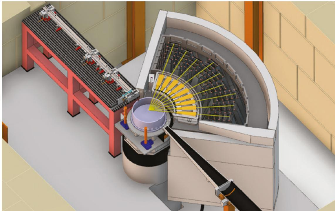
*BIFROST sample environment and novel prismatic analyser concept with efficient detector arrangement*
